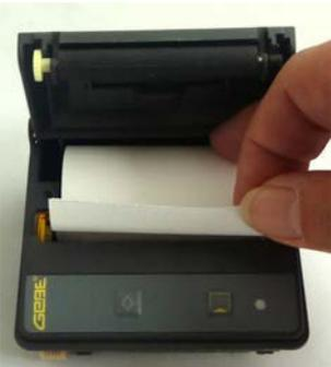
2. Unwind a few cm (inch) of paper from the roll. Keep the layers wound tightly when inserting the paper roll into the paper tray. The paper outside shows towards the printer mechanism.
