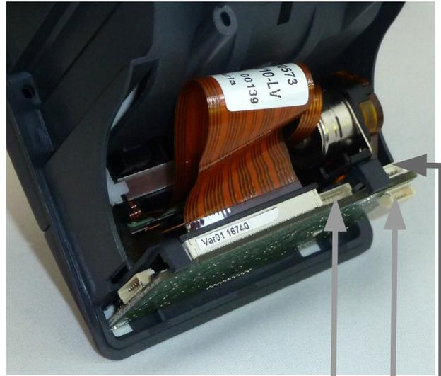
Figure 4: Controller board GCT-43611 LV version
