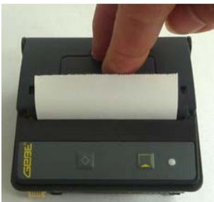
3. Close the paper tray by applying strong pressure. You can hear it snap shut. Now the paper can be torn off at the tear-off edge without opening the paper tray again nor the paper sliding through the printer mechanism.
