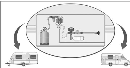
This test device can be used to check for leaks in accordance with the requirements:
