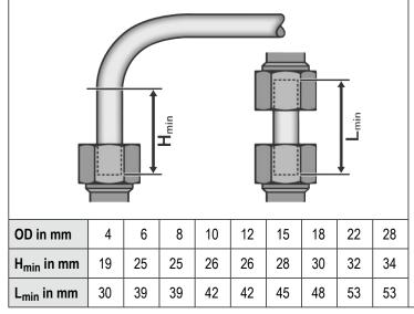
Table 5: Minimum length for straight pipe ends in pipe elbows H<sub>min</sub> and minimum length of straight pipes L<sub>min</sub>
